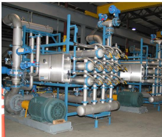
A KMS multi-stage amino acid crossflow microfiltration system equipped with eight-inch diameter housings for spiral wound membranes. Modular stages can be arranged to accommodate any production capacity and additional units are easily added for future expansion. Individual stages with Clean-in-Place design permit fast turnaround between production cycles.
